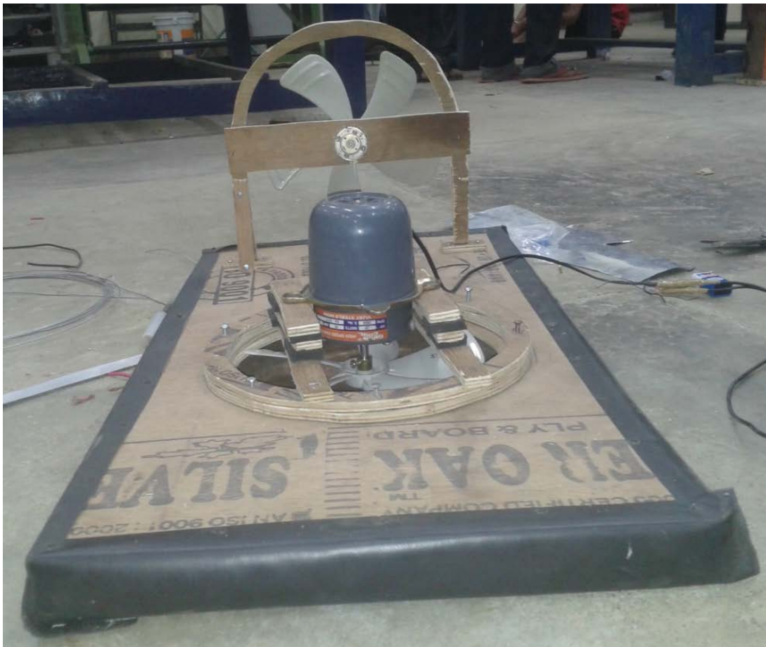
Fabricated model before installing Rudder, Microcontroller and Battery
