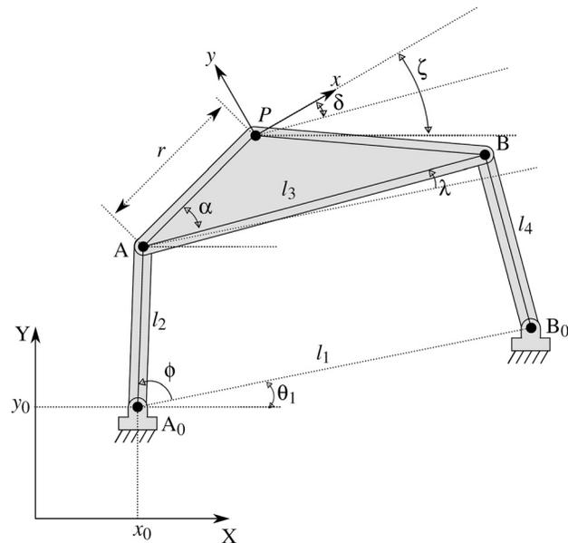
**Fig. 2** Visualization of parameters describing a four-bar mechanism
