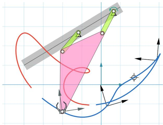
Fig. 8 Example 4: under-constrained mixed synthesis for three poses and one path points using additional motion constraint
