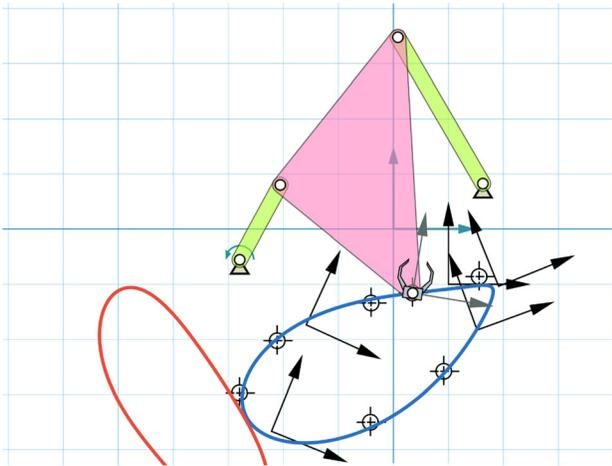
Fig. 4 Example 1: mechanism generated using mixed synthesis algorithm
